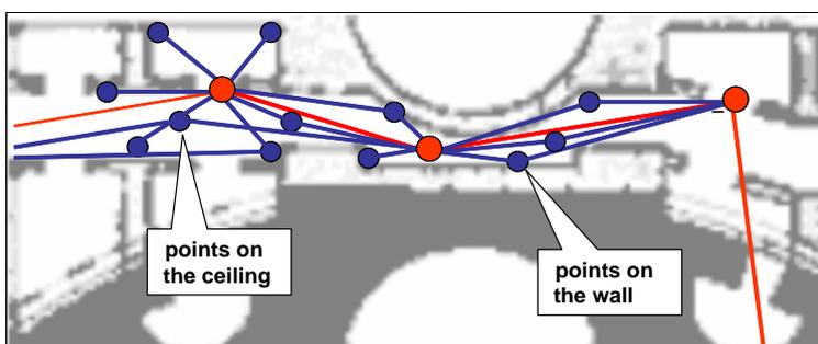
**fig. 1:** Object bound micro-networks replacing traverses (the red lines symbolise traverses while the blue lines symbolise the measurements to natural points at the walls or at the ceiling).
