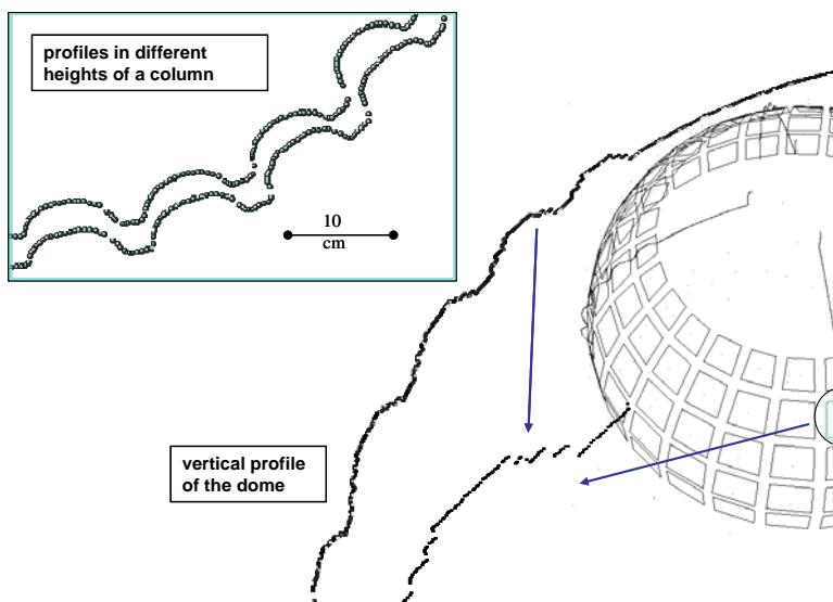
**fig. 7:** Horizontal (left) and vertical profiles (right) of high precision
