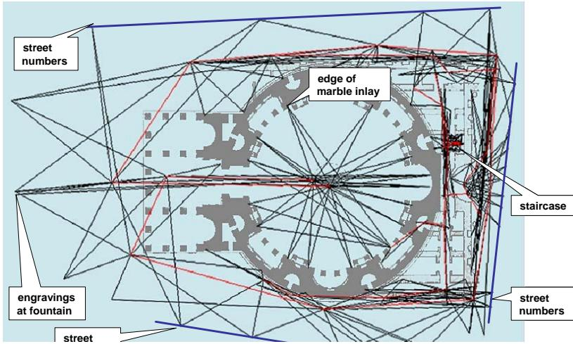
**fig.3:** Actual precise network of the Pantheon
