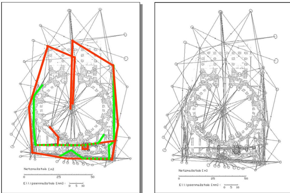
**fig 4:** Comparison of network accuracy obtained including traverses versus accuracy obtained using micro-networks alone
