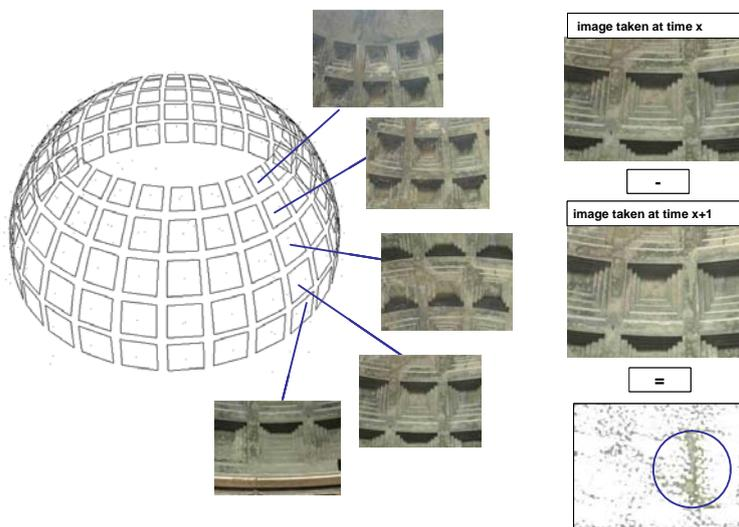
**fig. 10:** Demonstration of monitoring possible by differential analysis of images taken at different times
