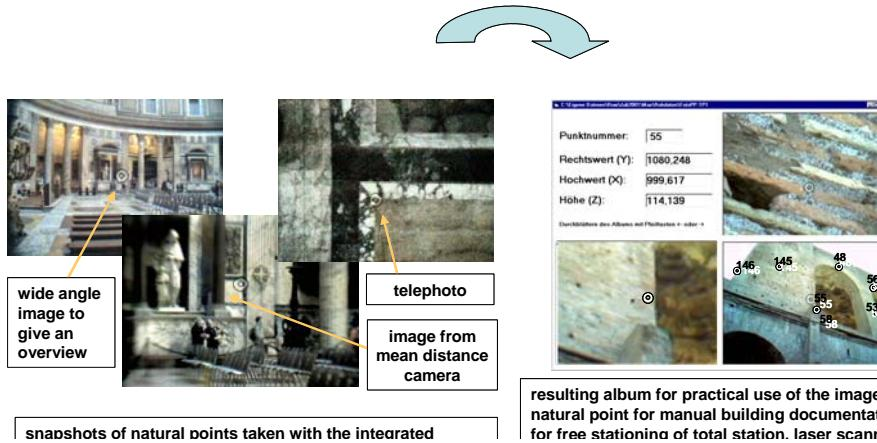
**fig.6:** Automatic documentation (from wide angle to telephoto) using a video total-station (left); album for the practical use of the images, i.e. for identification succeeded by manual measurements (right)
