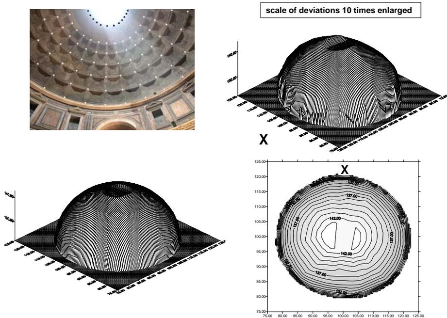
**fig. 8:** Analysis of the spherical form of the dome
