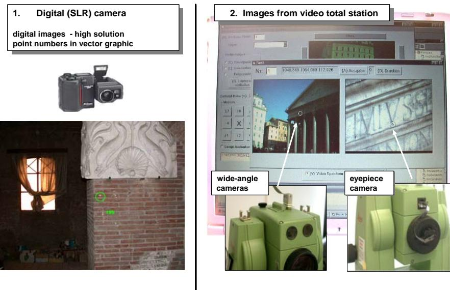
**fig.5:** Alternatives in documentation of natural points (left: with digital camera, right: using the cameras of the video-totalstation)
