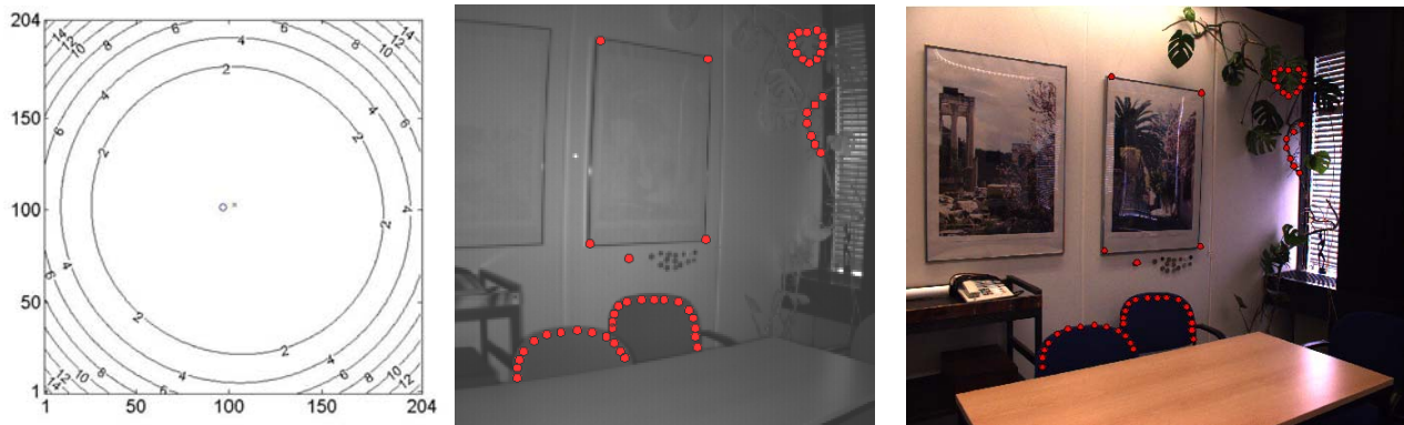
Figure 5: (left) Calculated distortion of the PMD-camera, (middle, right) Pixel transformation between PMD-camera and 2D camera.
